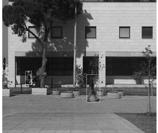
Figure 6 – Frame 440. CONDENSATION tracker segmentation results indicated by the two white bounding boxes. The person on the left with the white hat appears previously in frame 221 in a different orientation of his body.
