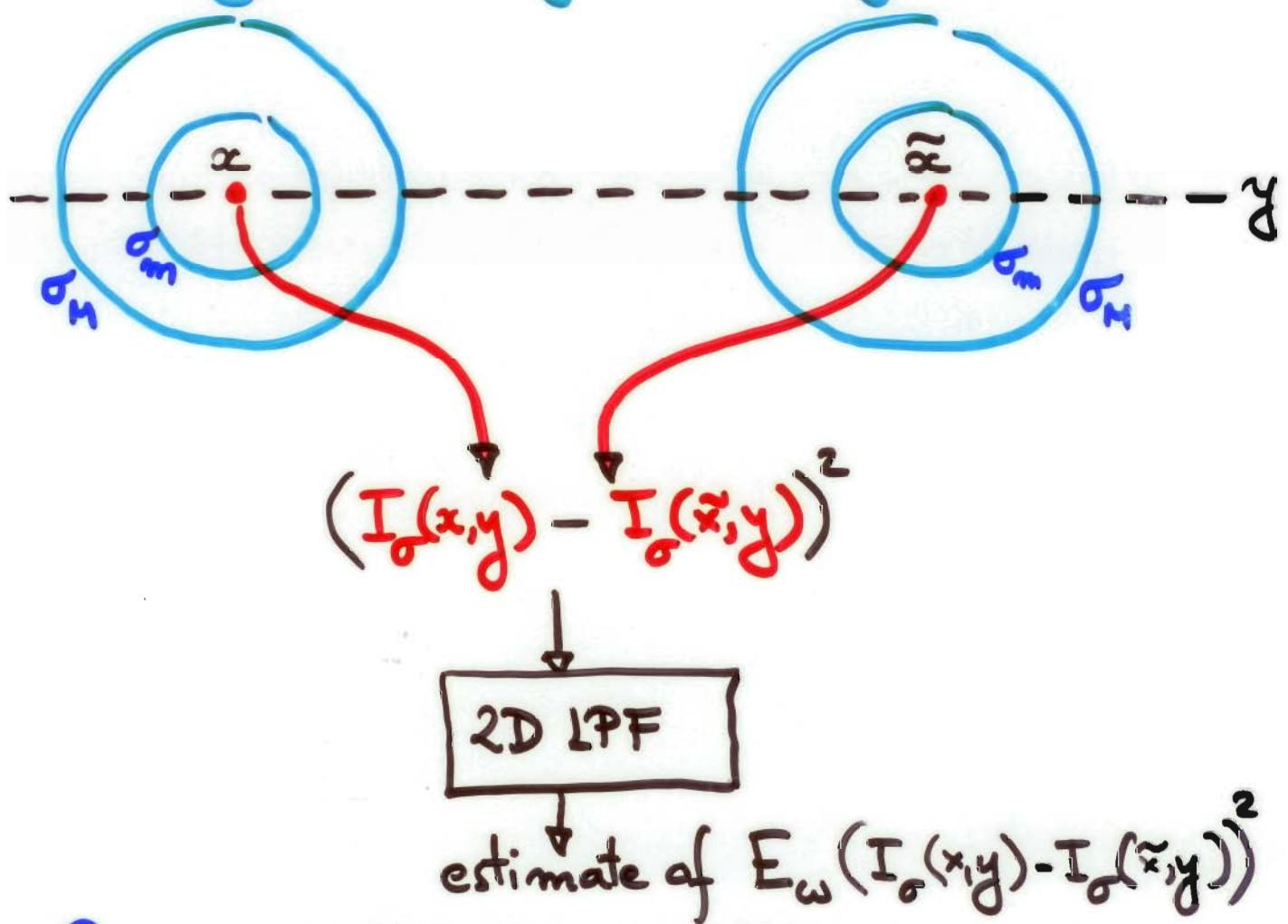
So we need to design  $I_o(x,y)$  so as to get the desired (1D) behavior for  $E_w(\cdot)$  here
