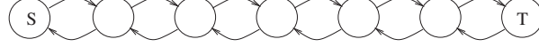
Fig. 2. All the agents are initially in vertex S of a chain-graph G , and all next-exit pointers initially point to the left. The motion is asynchronous; thus we let the next agent exit from S only when the previous agent arrives at vertex T . When all k agents are in T , the edge emanating from S was exited kD times, while the edge emanating from T was never traversed.
