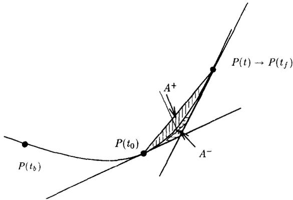
Fig. 3. An invariant parametrization using the area ratios.
