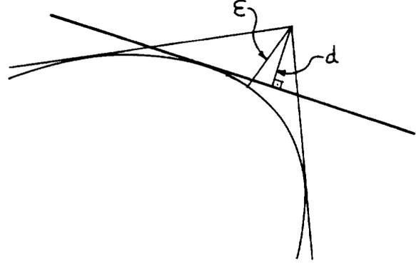
Fig. 12. Probing the true object with a line probe is equivalent to probing the circumscribing polygon with a positive error probe.
