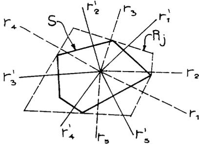
Fig. 8. A star diagram describing the probing process, the unknown object and the types of the vertices.
