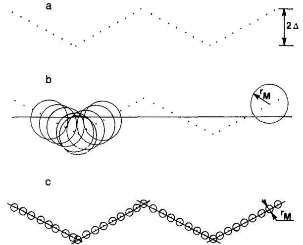
Fig. 3. (a) An arrangement of input points lying on individual line segments. (b)  $r_M$  is relatively large, thus the points are interpreted as lying on a single straight line. (c)  $r_M$  is sufficiently small, enabling the detection of the individual segments.
