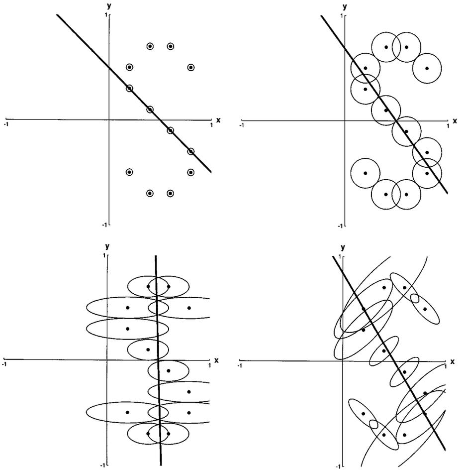
**FIG. 3.** (Top-left) Tuning the algorithm to compute the standard Hough transform. (Top-right) Robust TLS line-fitting. (Bottom-left) Robust heteroscedastic line fitting, without correlation. All points contribute to the fitted line, i.e., the saturation level is not reached in any point. (Bottom-right) Robust line fitting with heteroscedastic correlated noise.
