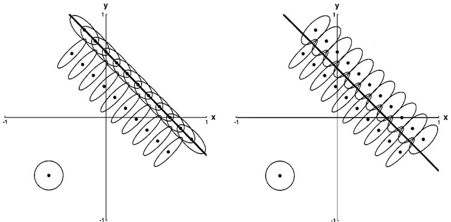
**FIG. 2.** Robust heteroscedastic line fitting with correlated noise. The differences in the records of the data points in these examples are only in the correlation values. (Left) The points in the smaller collinear group are regarded as outliers. (Right) The points in both collinear groups exert influence on the fitted line.
