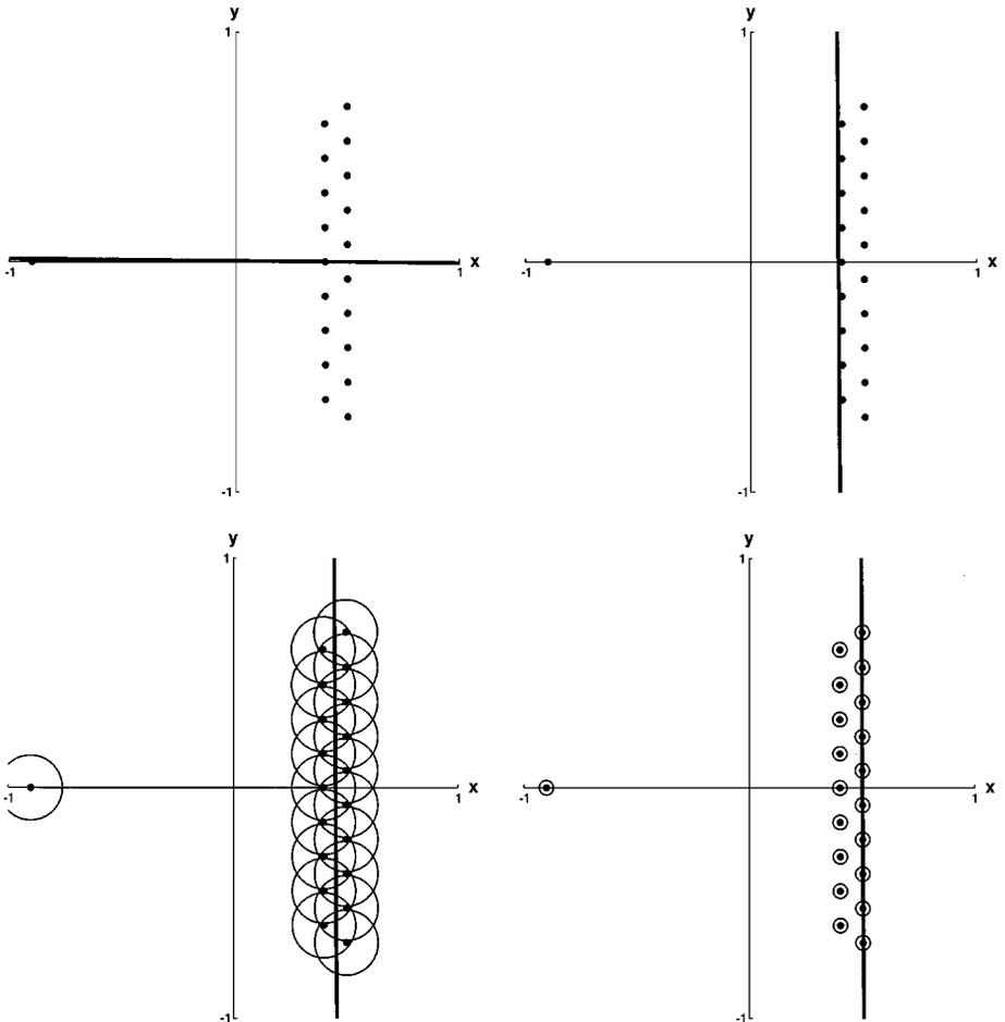
**FIG. 1.** (Top-left) Least-squares line fitting with errors in the  $y$  values only. The fitted line is horizontal. (Top-right) Total least squares (TLS) line fitting, as a special case of the suggested algorithm. (Bottom-left) Robust TLS. A data point has no influence beyond the circular contour. (Bottom-right) The standard Hough transform is obtained as a special case by setting the saturation level to a small value.
