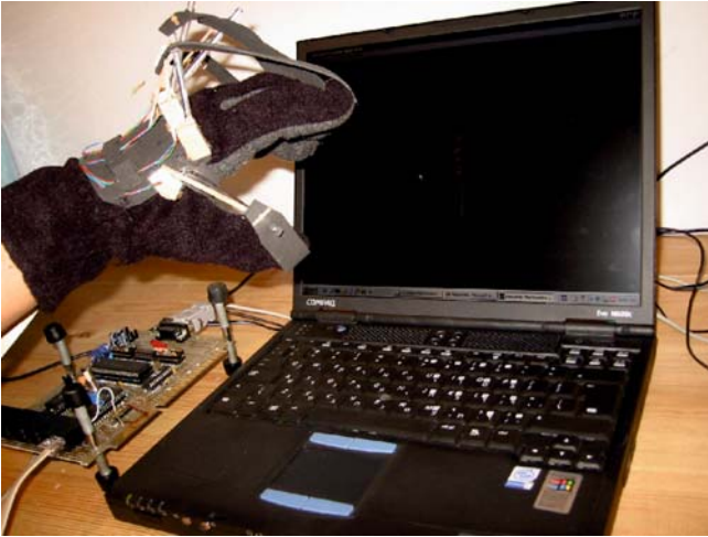
Fig. 1. A picture of one of the two data gloves that was designed and implemented as part of this project
