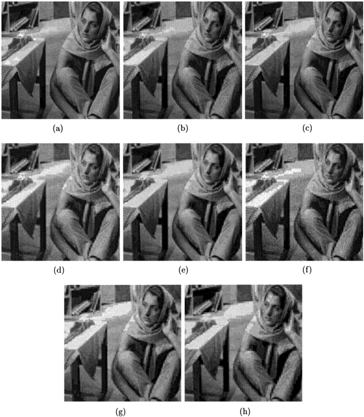
Figure 10. (a), (b) Best and worst images with randomized quantization and eight channels, total of 2 bpp. (c), (d) Best and worst images with four channels, total of 1 bpp. (e), (f) Best and worst images with two channels, total of 0.5 bpp. (g), (h) Best and worst images with one channel, total of 0.25 bpp.
