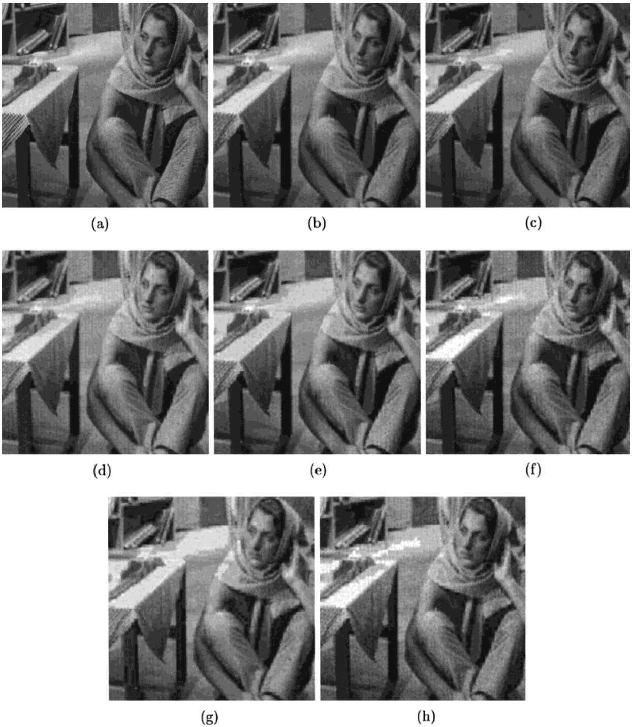
Figure 3. (a) Original test image of size 512 \times 512 . (b) Reconstructed image with eight channels, total of 2 bpp. (c), (d) Best and worst images with four channels, total of 1 bpp. (e), (f) Best and worst images with two channels, total of 0.5 bpp. (g), (h) Best and worst images with one channel, total of 0.25 bpp.
